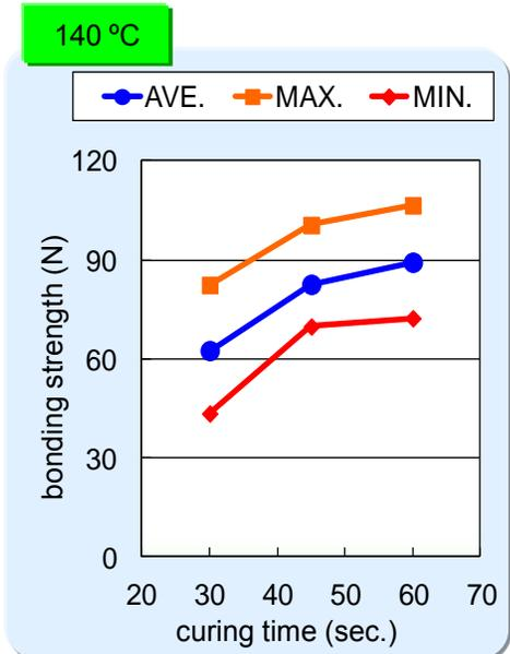
Recommended curing conditions: 1) At 120 °C for  $\geq 90$ sec. 2) At 130 °C  $\geq 60$ sec. 3) At 140 °C  $\geq 90$ sec.
