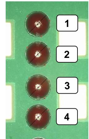
Change in diameter of the deposits after curing was only 5% in average and excellent heat slump resistance is secured.
